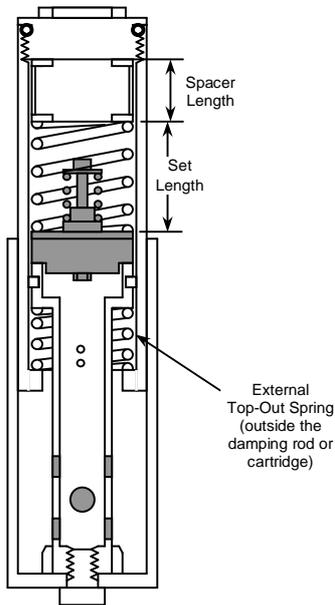
External Top-Out Spring (outside the damping rod or cartridge)
