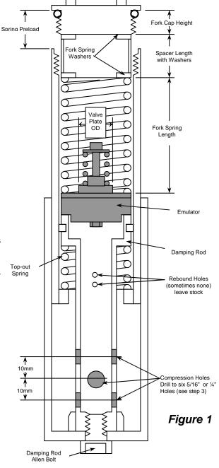
NOTE: If the bike is equipped with an Anti-Dive Mechanism or an External Compression Adjuster, the new holes should be drilled starting just above the Bottom-out Cones (or washers on models with washers). This will bypass the effect of the Anti-Dive but will result in a vastly improved ride. You do not have to disconnect the external Anti-Dive mechanism; it will be disabled with this modification.
