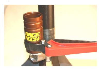
5. Install the RT Bladder/Cap assembly. Oil must overflow when the bladder is installed. Install the circlip.
